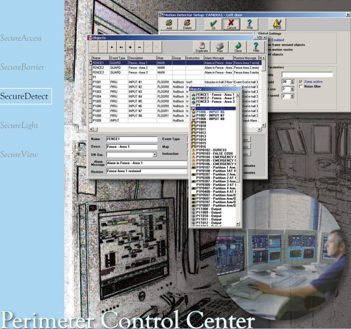
Safeguards Technology's Perimeter Control Center (PCC) is a security control system that processes data from various intrusion detection systems. After processing the data, the control center displays the information on a graphic display monitor. In addition to displaying the data, the center sounds alarms, issues messages, and displays alarm reports. The PCC is an advanced on-line tool consisting of a real-time software package installed on an IBM or compatible industrial computer.
